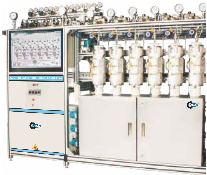
High throughput multi-tube reactor system for catalyst screening
