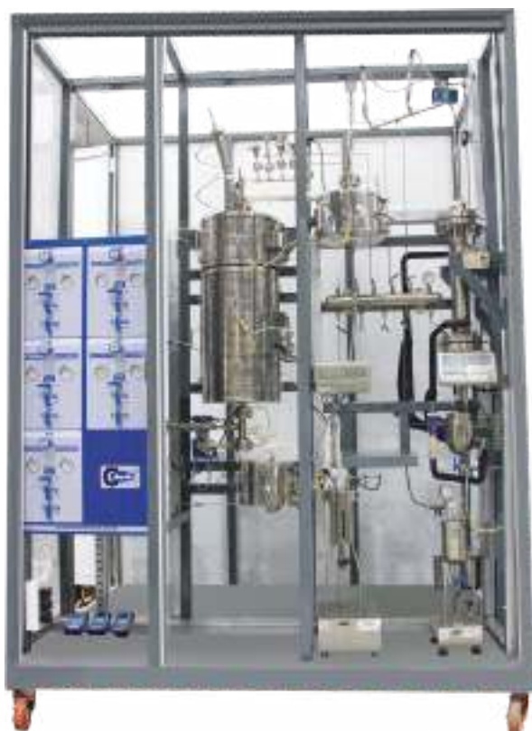
Fluidized bed reactor for fluidization of alumina
