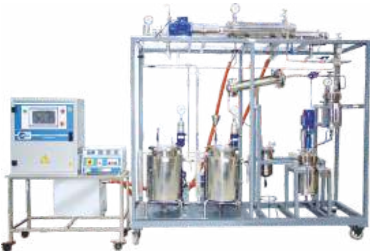
Hybrid pilot-scale setup of MACFLO™ & PinchFLO™ (2.5 L each) for Saponification with a throughput of 2 tons/day
